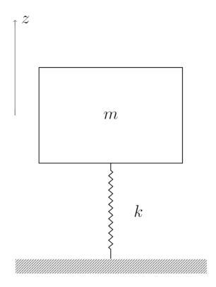
Analysis of the scheme allows to claim its number of degrees of freedom which is 1
